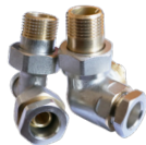
MASTER thermostatic valve, axial, left or right version. F 1/2" x M 1/2". Thermostatic head mounting thread M30x1,5. Economy version. Pre-setting. KN-01 setting key included. PEX version has a short PEX connector (16x2).
