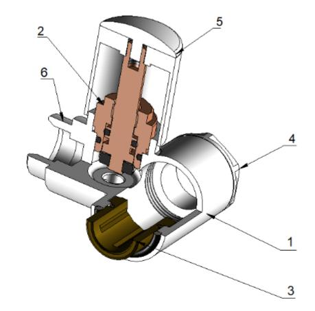
(\*) - standard connector is mounted on the PEX 16x2, it is possible to use the coupling for copper 15x1, or with an internal thread Rp  $\frac{1}{2}$  or external  $\frac{1}{2}$  G (type connectors selected ordering).
